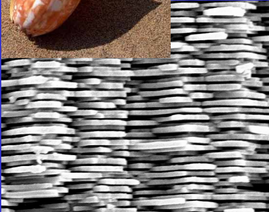
SEM images of cross section of nacre and chalk
